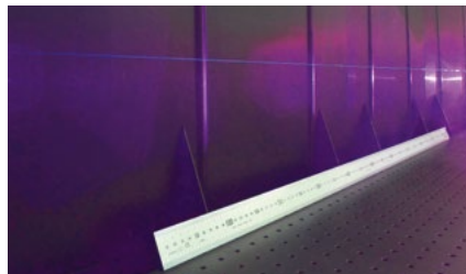
In atmospheric research, ultrashort-pulse lasers are used to create laser filaments in air. This technology enables triggering and guiding of lightning.
