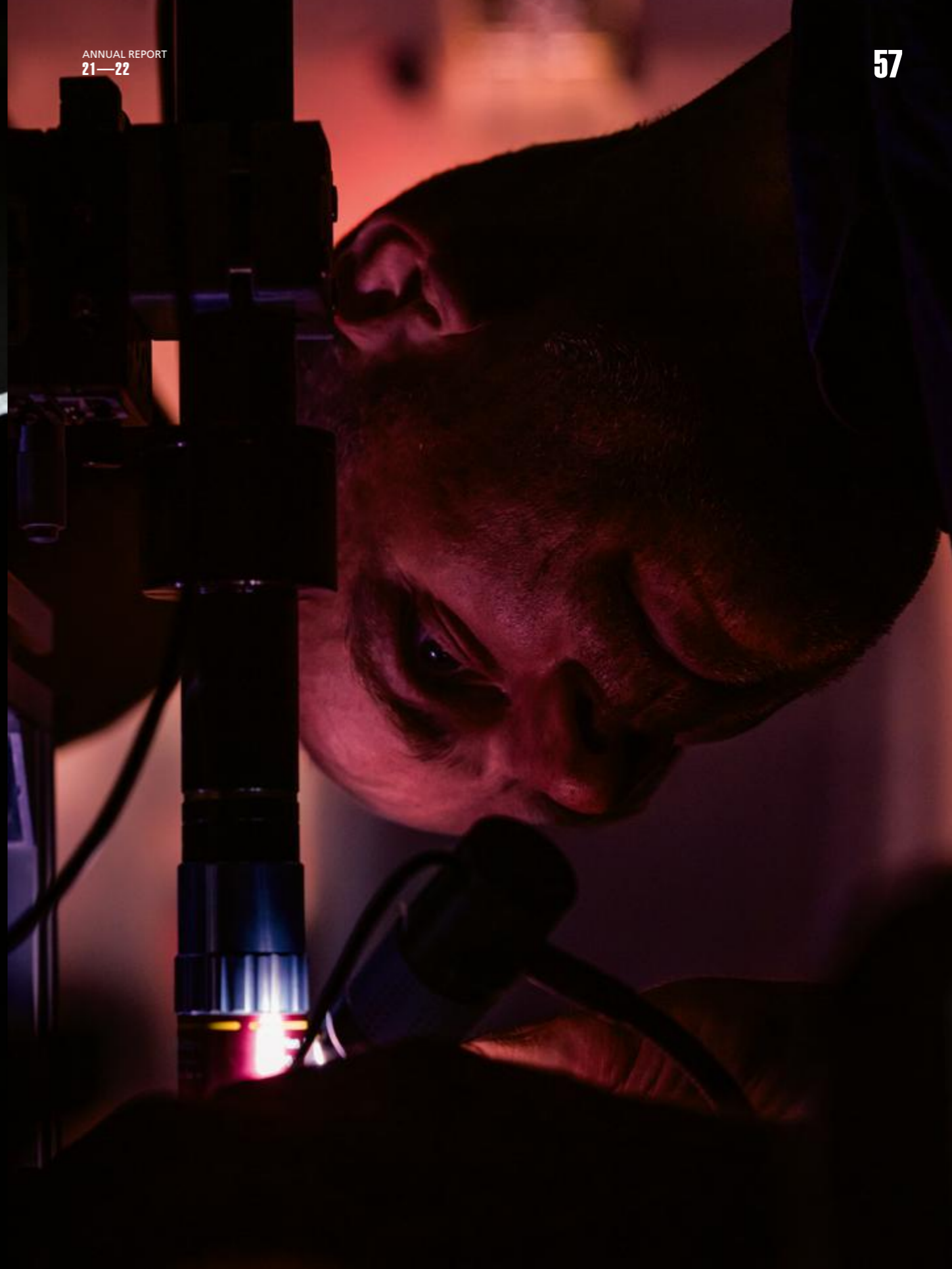
Victor Brasch sends light through a chip to test it.
