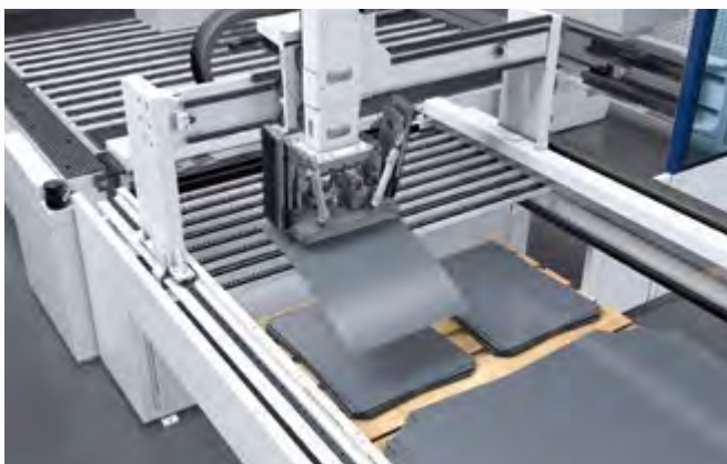
The suction gripper loads the TruBend Center 7030 automatically with large or small blanks while the machine is working.
