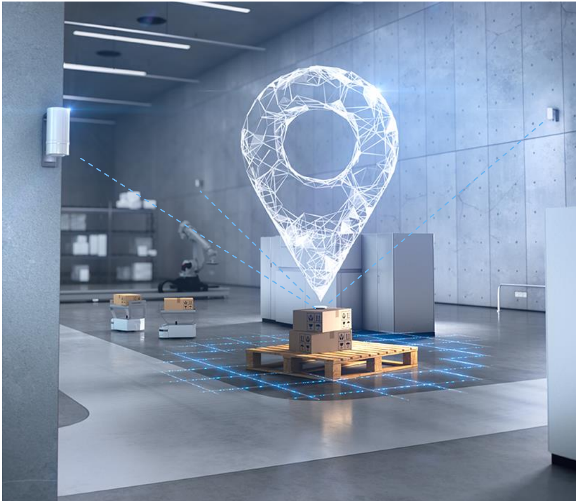
Figure 1: Typical industrial setup of an UWB-based RTLS consisting of fixed satellites and mobile tags to track objects
