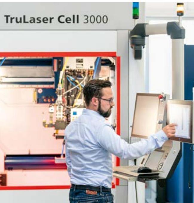
5_ René Schürer, team leader in the New Technologies division, operates a TRUMPF laser in a prototype system for hairpin stators.
