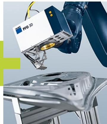
When used with scanner optics, the excellent beam quality of the fiber lasers enables both high processing speeds and large scanning areas.
