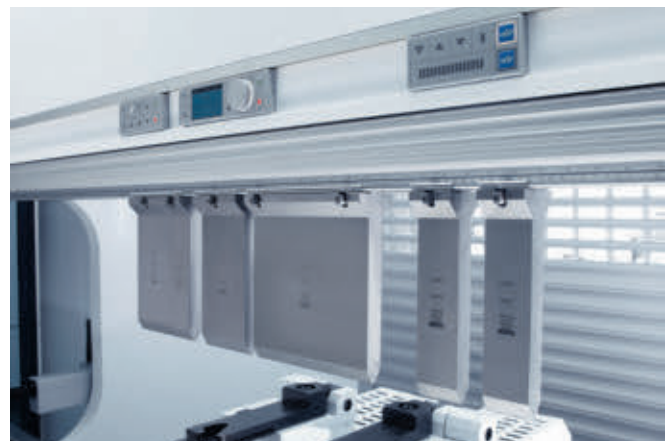
During set up the Tool Indicator shows precisely where the bending tools have to be used.
