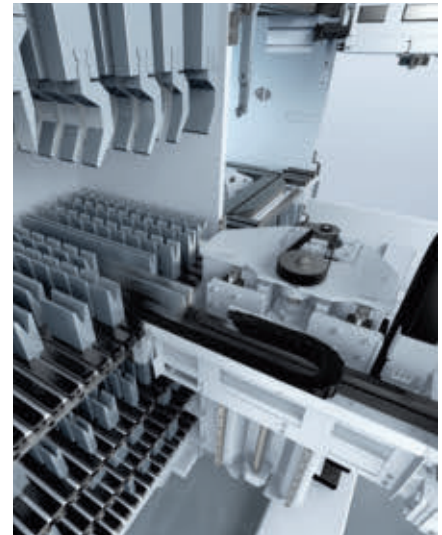
The ToolMaster is able to simultaneously load tooling segmentation into the rotary unit as the TruBend setup is being completed.
