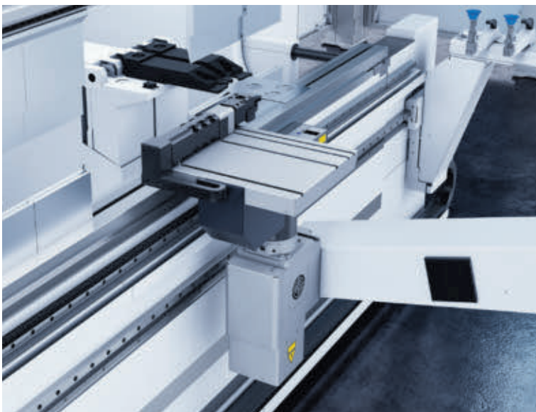
Pivoted-jaw gripper with moving and rotary axis
