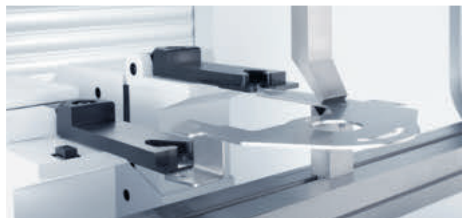
Flexible production due to 6-axis backgauge.
