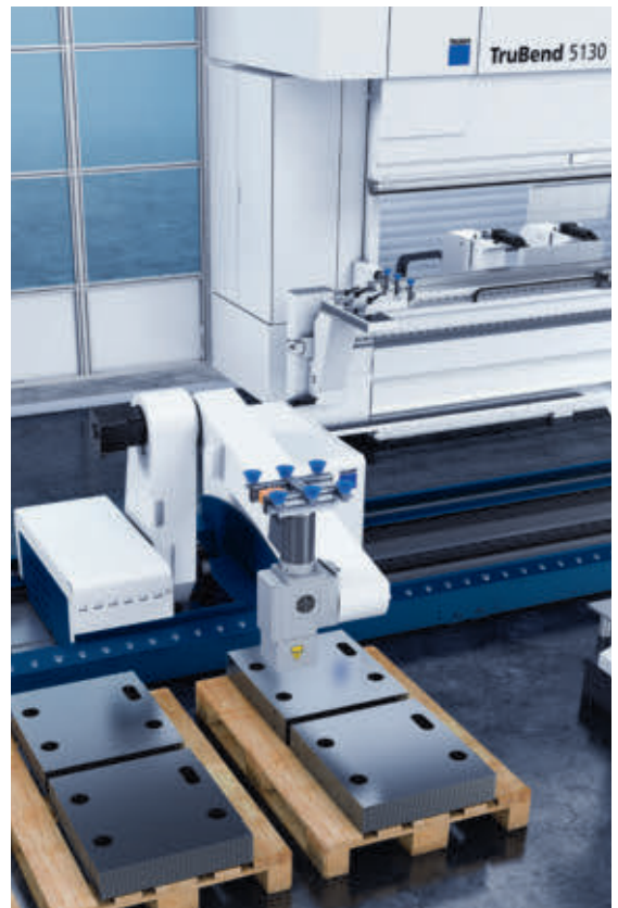
BendMaster (60) with fine-position recognition
