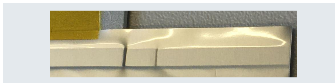
Figure 5: Process result with VCSEL heating system. Wrinkle free sealing at battery contact
