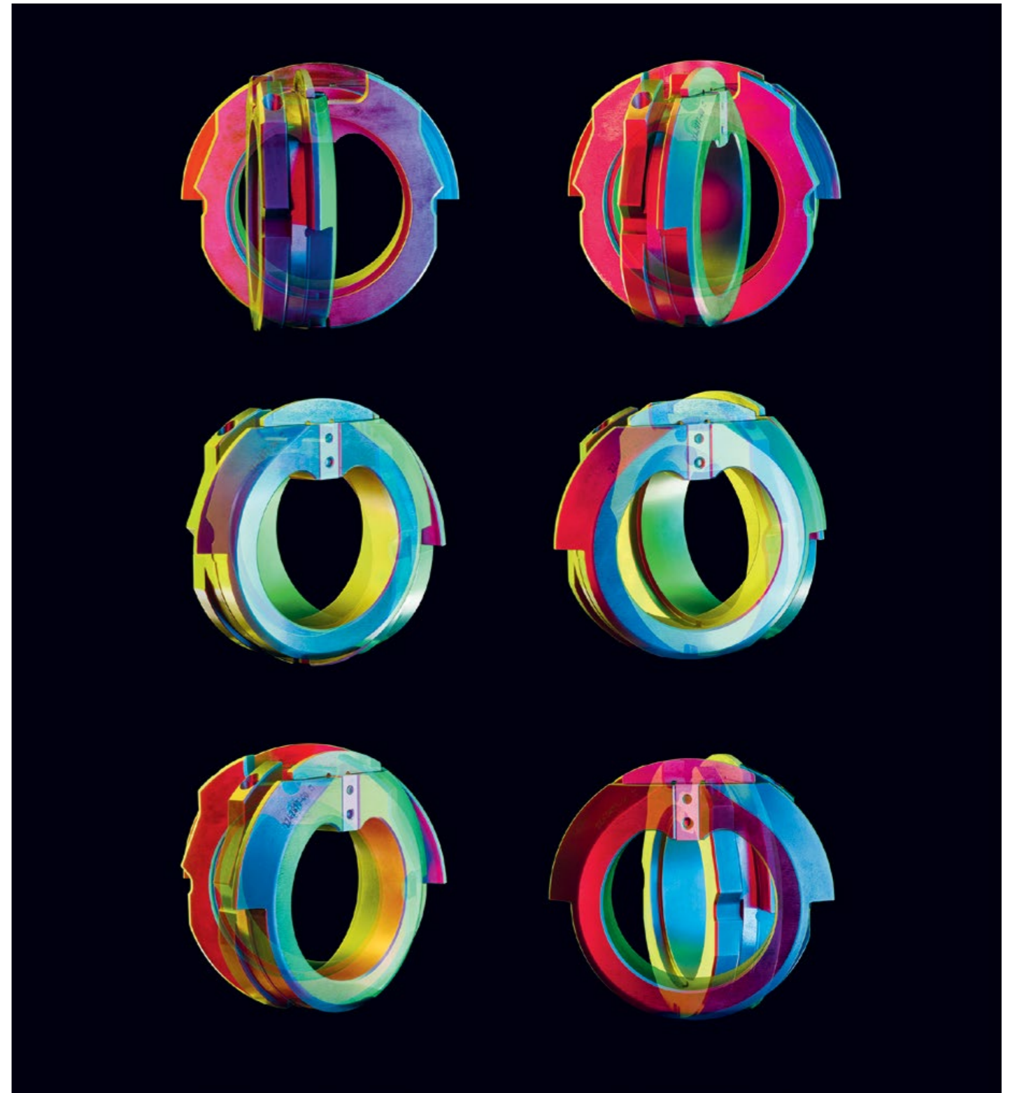
This picture shows a die for an ejector tool in a completely new light. The tool is used to sort parts in combination punch-laser machines. Using a series of targeted strokes, it removes laser-cut finished parts from the metal sheet and sorts them into "good" or "scrap" bins. Photographer Jan Kornstaedt has taken this tool out of its familiar environment and given it a whole new context.
