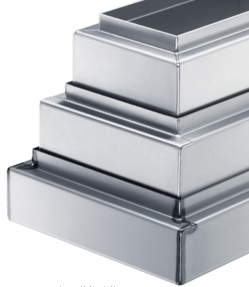
Laser welded terminal boxes (from bottom to top): mild steel, stainless steel, aluminum
