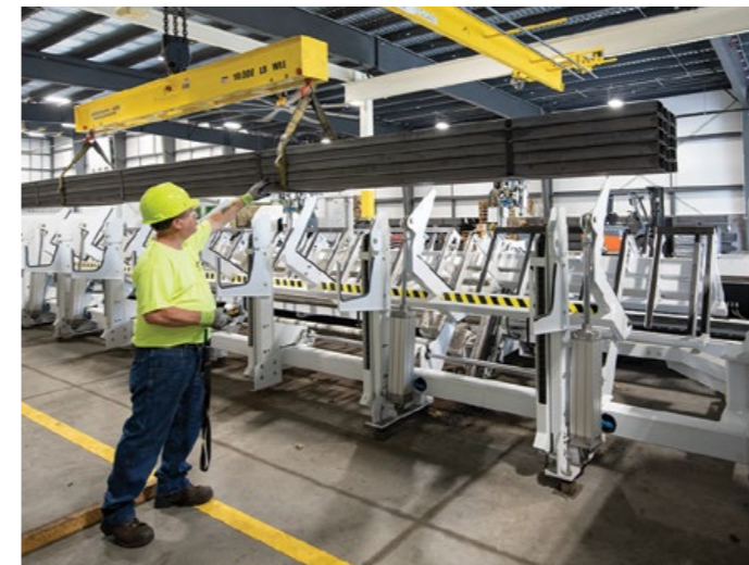
A Nitro Cutting employee loads raw material into the TruLaser Tube 7000 fiber.
