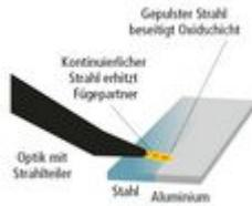
Aluminum and steel cannot be welded by conventional means. Using laser technology, however, makes it possible to create a solid lap joint. The laser fuses the steel in the focus of the beam, and the molten material heats up the aluminum beneath it. When it hardens, the steel forms a bond with the aluminum that is similar to brazing.
