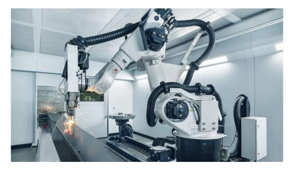
The TruLaser Weld 5000 large format machine at Böhmer Systemtechnik is equipped with a KUKA robot on a linear axis and a turnover positioner, allowing it to cover a working area 4 meters long and 1.5 meters wide. The rotate-and-tilt positioner gives users the flexibility to weld the occasional small part between a series of larger ones. © Günther Bayerl
