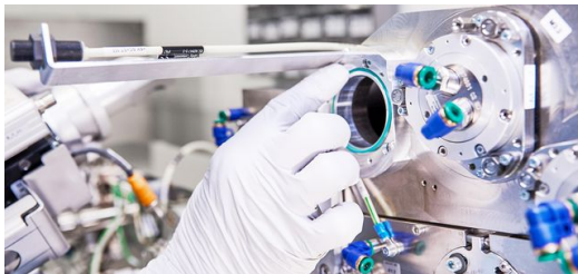
A mechatronics engineer installs a mirror mounting.
