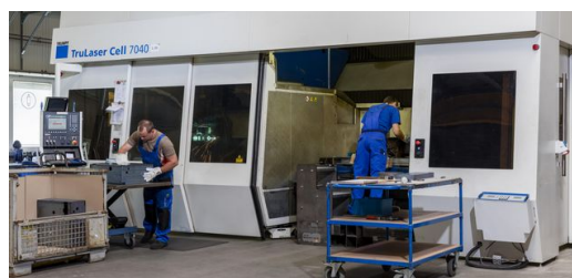
The TruLaser Cell 7040 manages visible seams of the best optical quality. The staff is able to make even complicated fixtures, ready for use within a week. Picture: Jan Gutzeit
