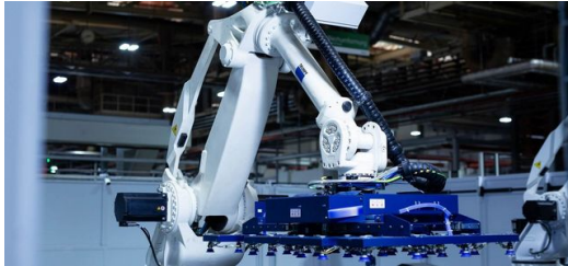
<p>The two unloading robots have their work cut out for them: The components come out of the laser cutting chamber in streams.</p>
