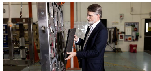
<p>The metal housings of the displays are mostly made of aluminum, with some parts made of steel. The actual display unit, the LED module, is embedded within them and connected to all the components in the system.</p>
