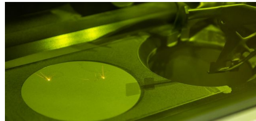
The pulsed laser in TRUMPF's TruPrint 1000 is an excellent choice for creating high-quality surfaces. Its multi-laser capabilities enable highly productive manufacturing processes. (Picture: Steffen Müller-Klenk)
