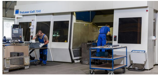
The TruLaser Cell 7040 manages visible seams of the best optical quality. The staff is able to make even complicated fixtures, ready for use within a week. Picture: Jan Gutzeit
