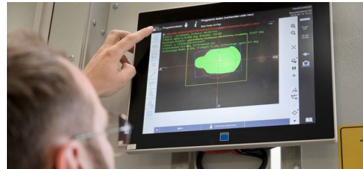
<p>The new AI filter option for VisionLine Detect enhances feature detection by creating a binary image of the part, i.e. displaying it in black and white only. This makes the welding areas stand out as sharply defined white surfaces.</p>
