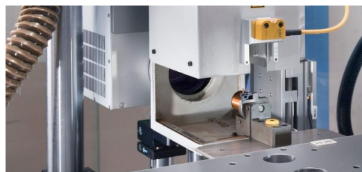
<p>The TruMark 5010 laser first removed the insulating varnish from the copper wire. The coil was then electrically contacted.</p>
