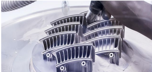
It takes just a few minutes to vacuum the excess powder off the part. (© Clauss Morgenstern)
