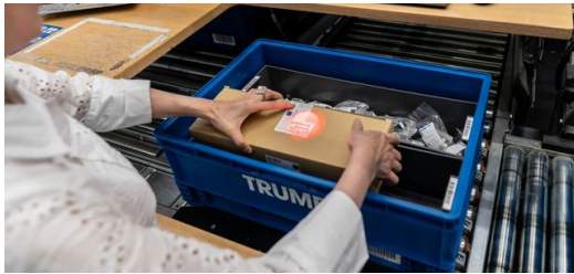
<p>Digital assistance: A coloured light marker directs employees on which components to place in each box.</p>
