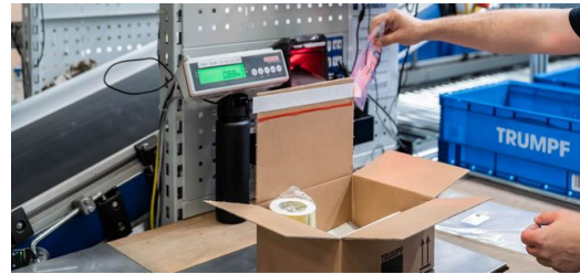
<p>Zero errors: Before dispatch, the employees check each parcel with an intelligent scale and compare the weight of the parts with the value stored in the system.</p>
