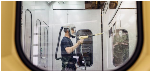
<p>The family-owned company also handles the powder coating of the housings itself.</p>
