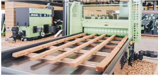
<p>Pallet chipper: Turns waste pallets into valuable biomass fuel.</p>
