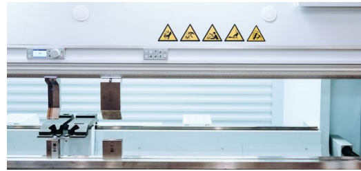
BendGuard: Safety instructions are always in the operator's line of sight. The BendGuard technology itself remains invisible, yet is capable of shutting the machine down in fractions of a second when necessary.
