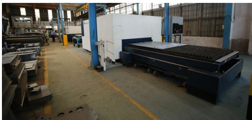
Lightweight doesn't always need high strength steels: JBM uses this TruLaser 1030 to produce profiles for buses.
