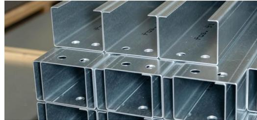
Precise product analyses by the SCHRAG project group show that some profiles exhibit a certain degree of standardization. In the future, these profiles will be produced automatically on a roll forming line at SCHRAG's Hamburg Seevetal site.
