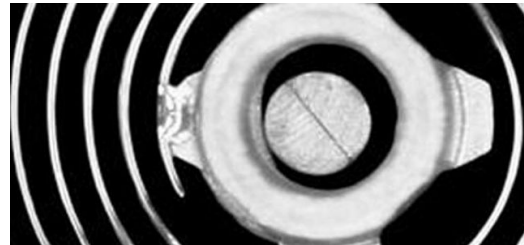
The welding spot has a diameter of 0.2 millimeters. Picture: TRUMPF
