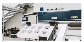
For boiler plate production, half-shell-shaped recesses must be made in the plate. First a hard nut for the TruBend Cell 5000. Today, the bending cell handles the forming process fully automatically, saving a lot of time.
