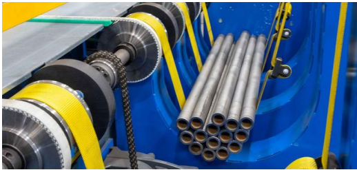
After cutting the tubes on the TruLaser Tube 7000, the tubes are transported to the production network where the robot places them in a bundle space and then distributes them on a table.
