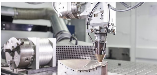
<p>The LMD process shown here on a TRUMPF system is suitable for repairing large parts and developing prototypes in the aerospace sector. (Source: TRUMPF / Claus Morgenstern)</p>
