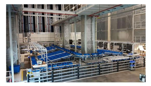
TRUMPF also relies on smart logistics. An automated small-parts warehouse whisks small spare parts to the packing station as if by magic.
