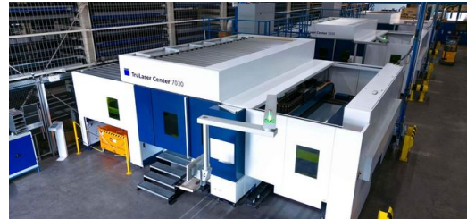
Automation and digitalization are the keys to success at VDL. The current installation of the three TruLaser 7030 full-service laser machines from TRUMPF aligns perfectly with this approach. They handle all laser cutting processes fully automatically.
