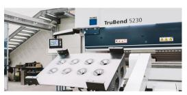
For boiler plate production, half-shell-shaped recesses must be made in the plate. First a hard nut for the TruBend Cell 5000. Today, the bending cell handles the forming process fully automatically, saving a lot of time.
