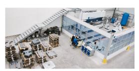
With its 230-tonne press force, the TruBend Cell 5000 can process components of  $3000\ x\ 1500$  millimeters conveniently.
