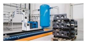
The processing of components with a weight of 60 to 80 kilograms are the order of the day at PNH. To promote the health of his employees, Martin Mitterhumer has equipped his installation with vacuum grippers and pivoted-jaw grippers.
