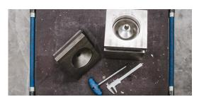
The special tools developed by TRUMPF in Pasching especially for PNH, enables to automate the rigging of semicircular, bowl-shaped depressions required for the boiler plate manufacturing process.
