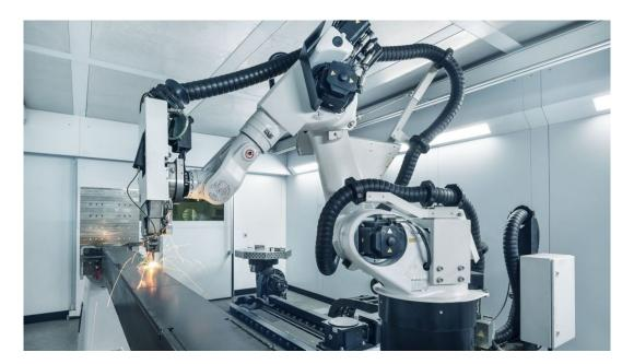
The TruLaser Weld 5000 large format machine at Böhmer Systemtechnik is equipped with a KUKA robot on a linear axis and a turnover positioner, allowing it to cover a working area 4 meters long and 1.5 meters wide. The rotate-and-tilt positioner gives users the flexibility to weld the occasional small part between a series of larger ones.
