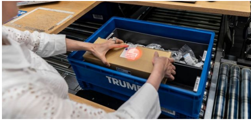
<p>Digital assistance: a colored light marker shows employees which components they should place in which box.</p>
