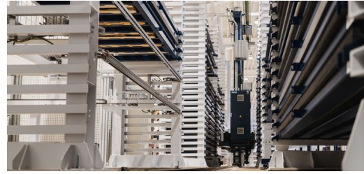
The large-scale storage system: STOPA is fully automated and sends the sheet metal material on its production journey and retrieves the finished parts just as efficiently.
