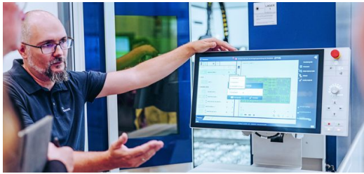
Control panel: Demonstration engineer Uli Schrade shows how every safety parameter is clearly visible on the display before the laser can start.
