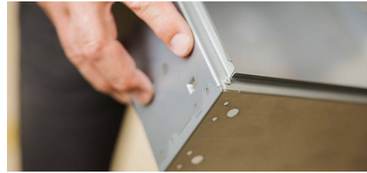
<p>Max Knobloch can even perform small forming operations, such as cup embossing or clip connections, with the TruMatic 7000.</p>
