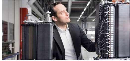
Up to 400 bipolar plates are stacked alternately with membrane assemblies to form a fuel cell.
