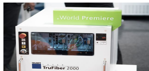
The fiber-based solid-state laser TruFiber 2000 celebrated its world premiere at the LASYS 2018. Because this laser has a compact laser design, flexible interfaces to all common fieldbus systems, and the maximum laser safety rating with Performance Level 'e', it also contributes to easy integration. Image: Lorenz Buchwald
