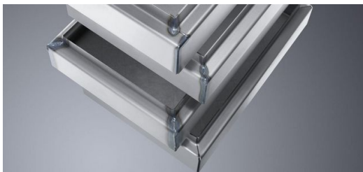
Mild steel terminal box (from bottom to top): unwelded, manual MAG weld, FusionLine weld, and laser weld after redesigning for laser processing. (Picture: Oliver Graf Fotostudio GmbH)
