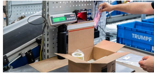
<p>No errors: before dispatch, the employees check each parcel with an intelligent scale and compare the weight of the parts with the value stored in the system.</p>
