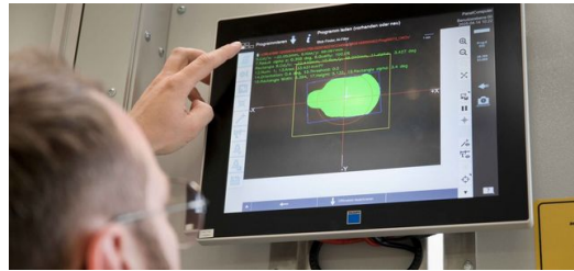
<p>The new AI filter option for VisionLine Detect improves feature detection by binarizing the component - i.e. displaying it in black and white only. The welding areas stand out as sharply contoured white areas.</p>
