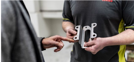
<p>Every component meets the most stringent quality requirements. After bending, the parts are robot-welded, so the tolerances are correspondingly tight, at plus or minus 0.25 degrees.</p>
