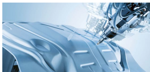
EdgeLine Bevel enables bevels that prevent deposits from forming at the edges of the weld. As a result, the components lose weight.
