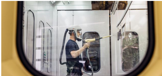
<p>The family-owned company also powder coats the housings in-house.</p>
