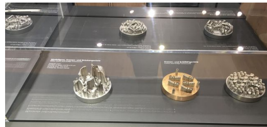
Substrate plates with 3D-printed dental prosthesis.
