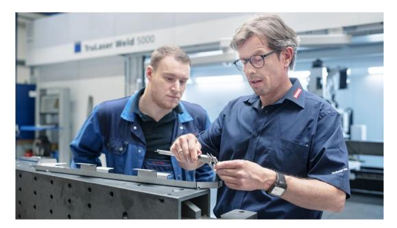
Deep penetration welding with a laser involves far less heat input than conventional welding methods – and that means less distortion. Josef Böhmer (right): "Parts nowadays have to be made to such fine tolerances, especially in formwork construction. So we save a lot of time by not having to straighten them after welding!
