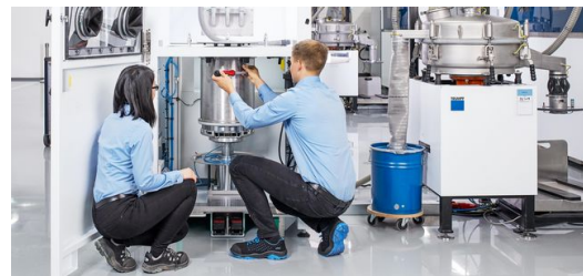
The construction cylinder is mounted in the unpacking station. (© Claus Morgensern)
