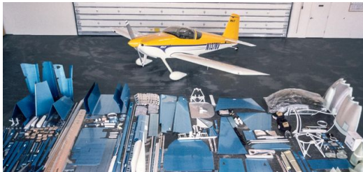
Van's Aircraft delivers knocked-down airframes as individual components in several conveniently sized boxes or crates. Hobby pilots all around the world put them together. (Picture: Van's Aircraft)
